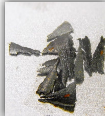
1.5 = One spot to 20% corroded
