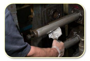
62 RP SPINDLE LUBE is cleaned or removed using any common petroleum hydrocarbon solvent, such as kerosene or mineral spirits.
