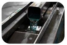
**2200 LX CHARCOOL**: AMCOL's premier coolant package. Used where severity of forming requires high lubrication to prevent galling and pick-up. This coolant contains special additives to provide enhanced rust protection and biostability.
