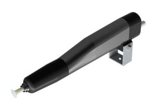
Produces an electrostatic field which allows the release agent to stick to the grounded billet. Comes standard with a 20mm deflector cone (12" billet or under) which provides a light, round spray pattern with uniform film thickness. 28mm and 38mm deflector cones are also available for larger billets
